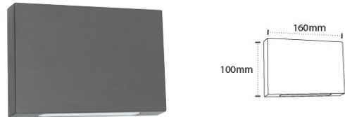
AL 333 - 2x6W Color Temperature : 3000K, 6000K Material: Die-casting Aluminium with PC Diffuser Body Color: Graphite Gray
