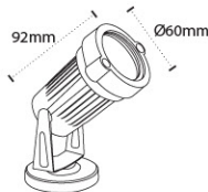
AL 4095 Wall Light LED: 5W Holder: GU-10, MR-16 Color Temperature : 3000K, 6000K Material: Die-casting Aluminium, Metalised Reflector with Toughened Glass Body Color: Black
