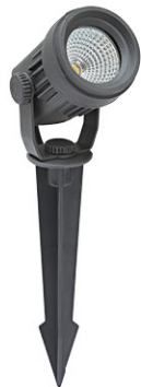
AL 5100 - 7W Color Temperature : 3000K, 6000K Material: Die-casting Aluminium, Metalised Reflector, Toughened Glass with ABS Spike Body Color: Graphite Gray
