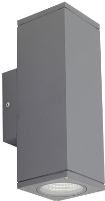
AL 2610 - 2 Color Temperature : 3000K, 6000K Material: Die-casting Aluminium, Toughened Glass with Metalised Refletctor Body Color: Graphite Gray
