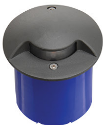
Cut Size: Ø75 x 70 mm AL 4050 - 1x1W Color Temperature : 3000K, 6000K Material: Die-casting Aluminium, PC Diffuer with ABS Recess Box Body Color: Graphite Gray
