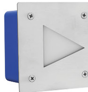
AL 3910-C - 4W Color Temperature : 3000K, 6000K Material: Die-casting Aluminium, S.S. 304 Grade Laser cut Plate, PC Diffuser with ABS Recess Box Body Color: Steel Finish
